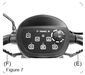
**Lighting** – All CTM scooters come with lighting packages. It is recommended to turn these lights on when the scooter is in use. The Medium and Large models come with indicators. These will beep loudly when in use. The beep can be turned down or off by your local dealer.
